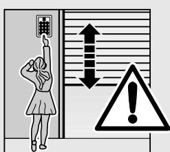
**Permanently installed controls (such as buttons or similar devices) should be installed within sight of the door but well away from any moving parts. It is vital that they are installed well out of the reach of children at a height of at least 1.5 metres!**
